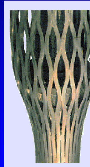
Alternative Borehole Liner
